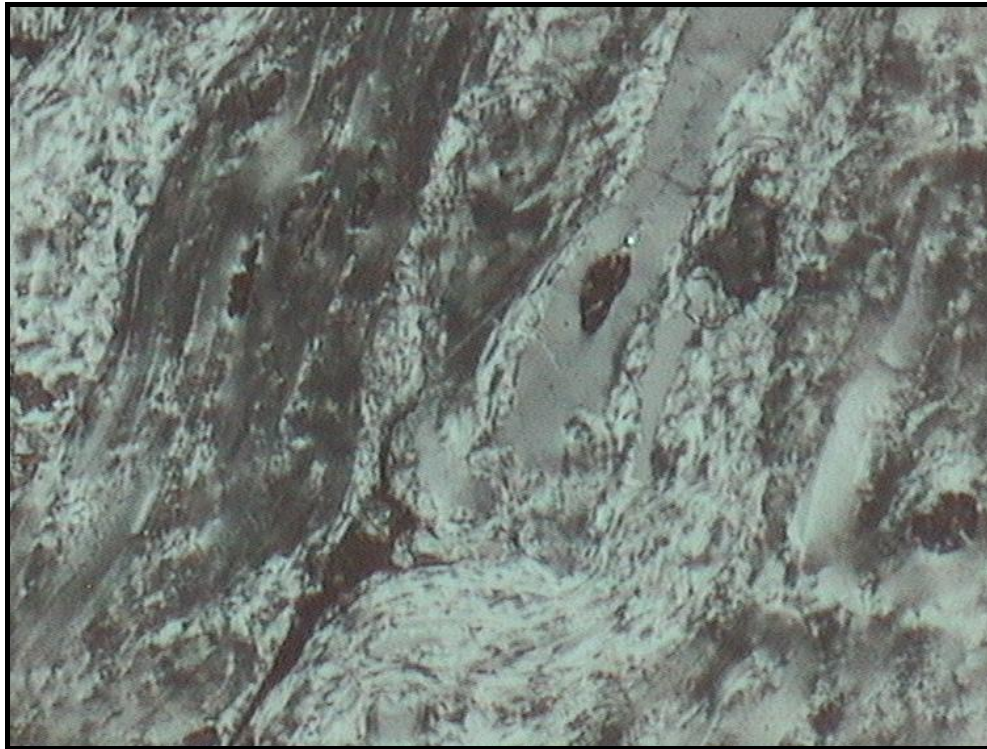
Figure 3.11. Semi-coke in Bowen Seam coal, Bowen No.2. Pit. Sample Number BO3.61-4.21. Field of view 50 \mu\text{m} wide. Polarised light.
