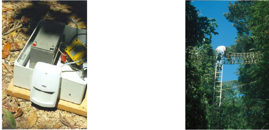
Figure 4.6a, left, Data logger ( Tinytag Plus ) attached to an infrared detector, enclosed within a weatherproof case and powered by a 12-volt rechargeable battery; b, right, A 3-section extension ladder was used to access the logger to download data to a laptop computer (Photo: Steven Nowakowski)
