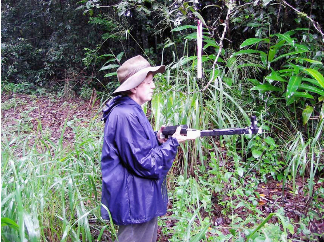
Plate 4.3. The red:far red sensor and display meter were supported on a flat wooden post. The sensor and a level bubble were placed at the far end of the post, to avoid being shaded by the operator. The instrument was held at chest height (~1.3 m above the ground surface) and measurements were taken only on overcast days with uniform light conditions. The person pictured is June Pohlman. Photo by author.
