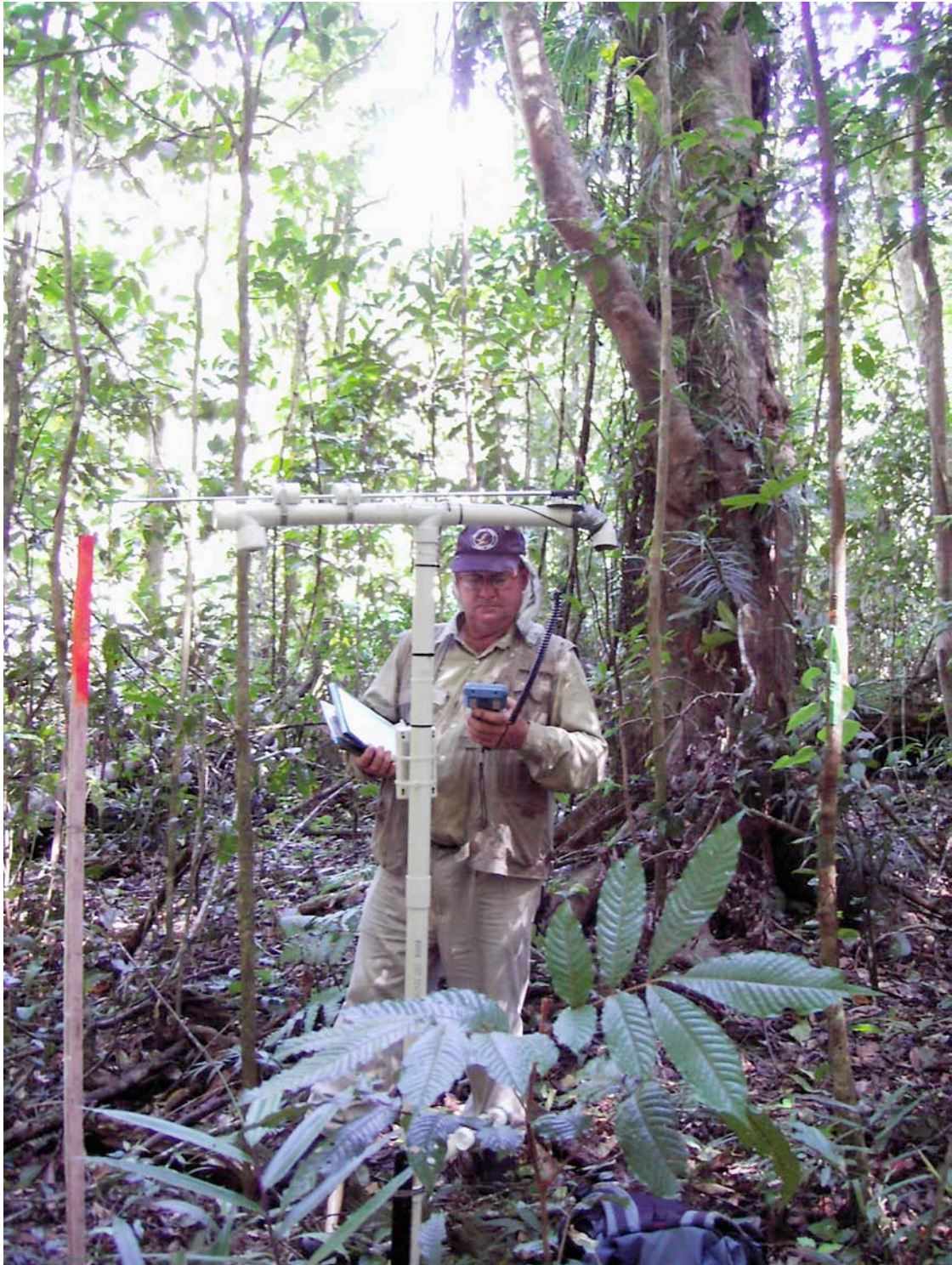
Plate 4.1. The instruments used for the traverse measurements were supported on a PVC frame. The quantum sensor was attached to the top of the frame (on a leveling mount). Two “arms” were placed at heights of 165cm and 30cm, with supports, to hold the hot-wire probe. As the hot-wire probe was sensitive to very slight movements, the entire frame was slotted into a second, supporting frame that was clamped to a star picket which was hammered into the ground at each measuring point. This allowed the frame to be free-standing and avoided confounding measurements of air speed with inadvertent hand movements from a person holding the frame. The person pictured is Stephen Pohlman, who is holding the display meter for the hot-wire probe. Photo by author.
