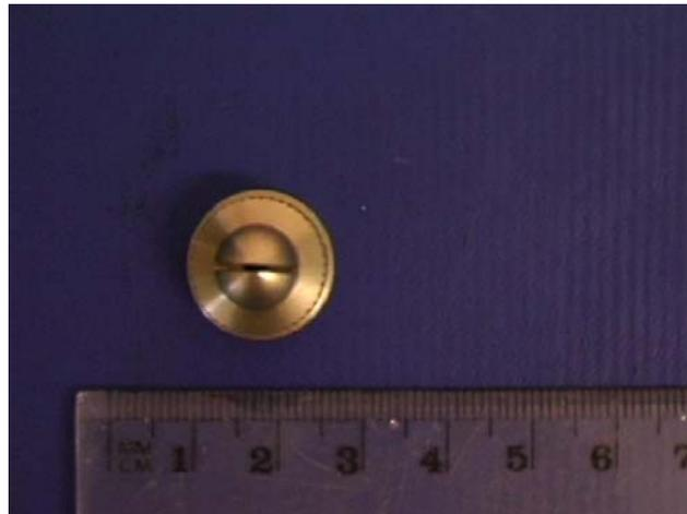
Fig. 3.9 A and B. Spraying combination: Head bore orifice 2 mm bore (A) and nozzle cap 3.5 mm bore/ 0.95 mm gap split nozzle cap (B).
