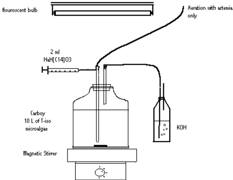
Fig. 2.3 The apparatus used to label *T-Isochrysis* sp. (*T-iso*) microalgae and *Artemia*. The apparatus was under constant illumination.
