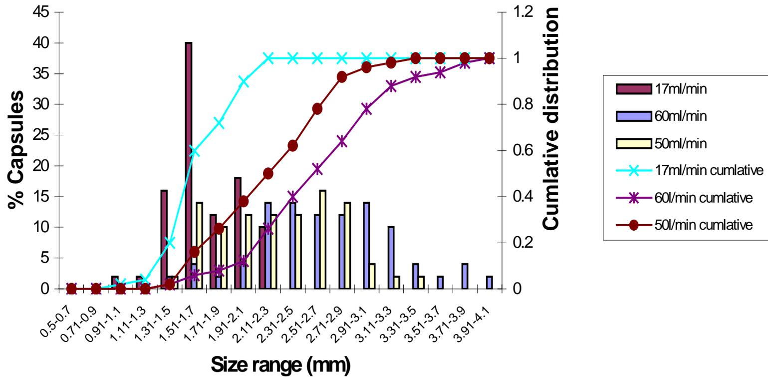
Fig. 4.6. The size frequency distribution of complex MC produced using Treatment 1; using 3 different flow rates of dietary material, without a mechanical device and with needle gauges of 21G inner: 16 G outer.
