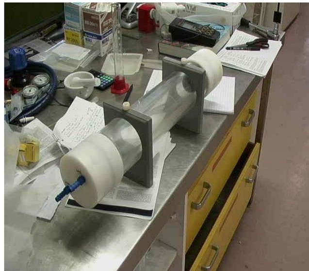
Fig. 3.3 (A and B). The sprayer device and dietary cylinder used to prepare sprayed beadlets. A, the atomisation apparatus with heated water jacket from Spraying Systems Co. and the dietary cylinder B, which is N<sub>2</sub> piston driven and heated to desired temperature of 35°C by surrounding water jacket. (Sourced and further modified from D.F. Villamar and C.J. Langdon, 1993; C.J. Langdon pers. comm, 2001).
