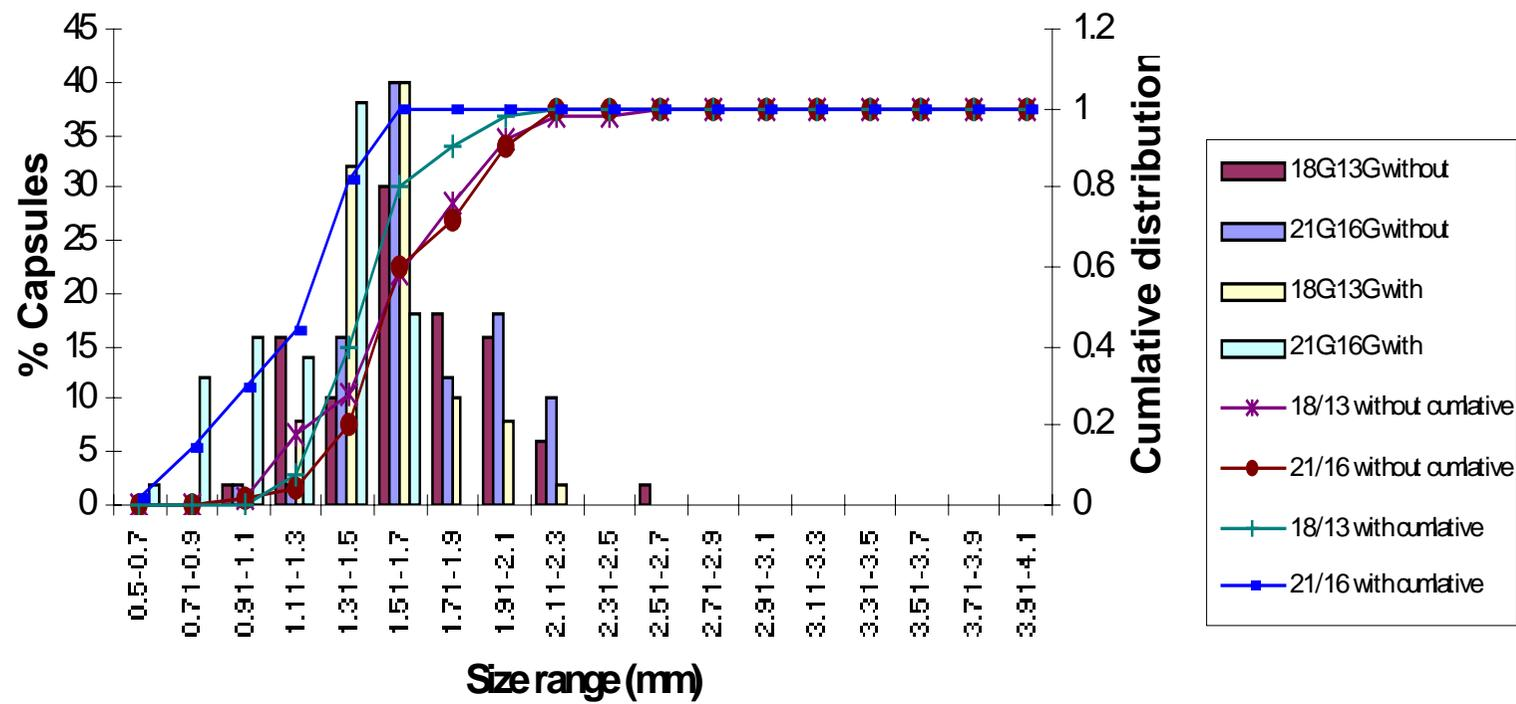
Fig. 4.8. The size frequency distribution of complex MC produced using Treatment 3; using different needle diameter combinations (Flow rate of 17 mL/min).
