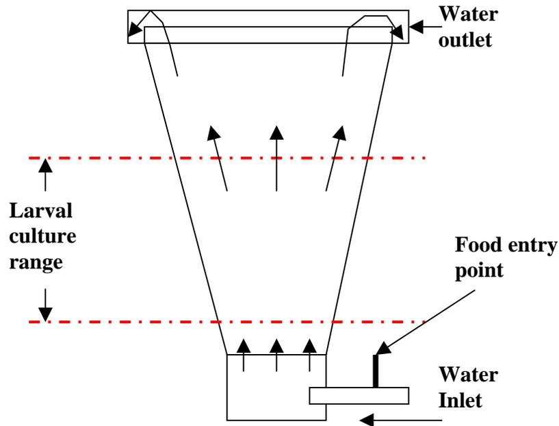
Fig. 3.10. The up-welling larval culture tank used for *P. ornatus* phyllosoma. The preferred larval culture depth range for phyllosoma is indicated. The filtered seawater travels through the adjustable water inlet then through a porous plate forming vertically laminar flow.
