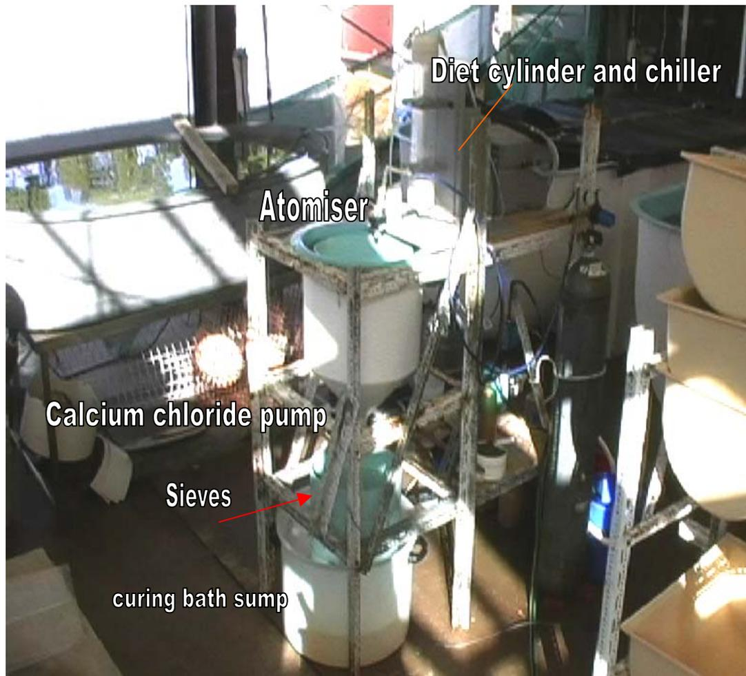
Fig. 3.6. The spraying tower used to produce sprayed beadlets (side view). (Note the recirculating  $\text{CaCl}_2$  curing bath (75 L) with sump containing desired sized stackable sieves  $>850, 500, 355, 210$  and  $100 \mu\text{m}$ ).
