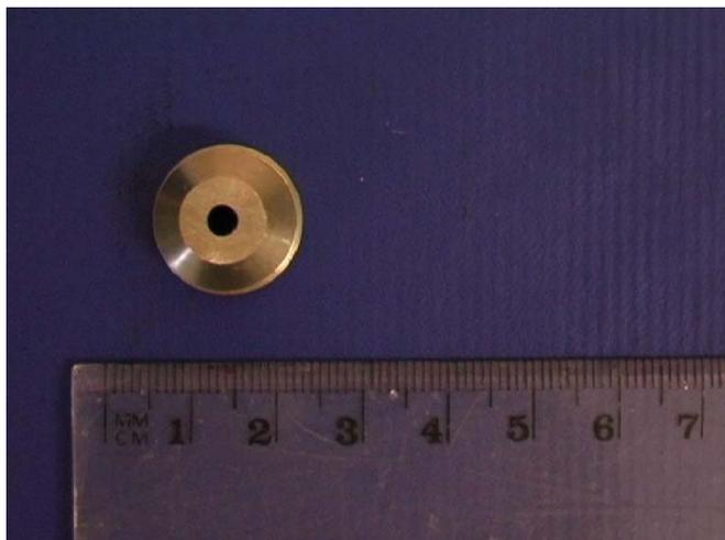
Fig. 3.7 A and B. Spraying combination: Head bore orifice 2 mm bore (A) and nozzle cap 3.5 mm bore (B).
