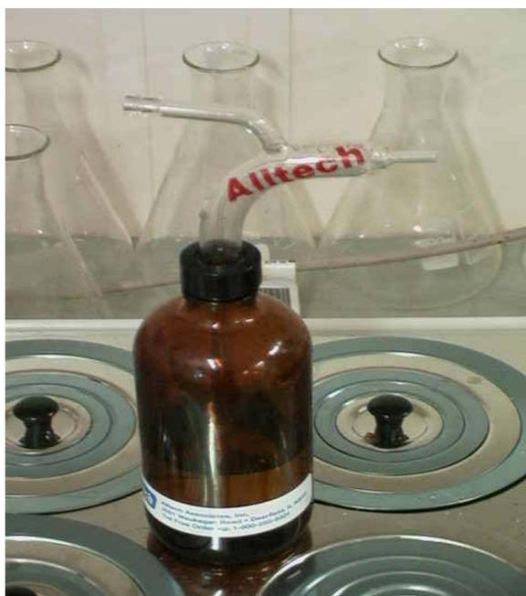
Fig. 3.1 (A and B). The Alltech Inc. hand held glass atomisers. A, Apparatus used for production of fine particles and B, Coarse particles. The atomisers each held 250 mL. The diet mixture can be preheated within a water bath prior to spraying.
