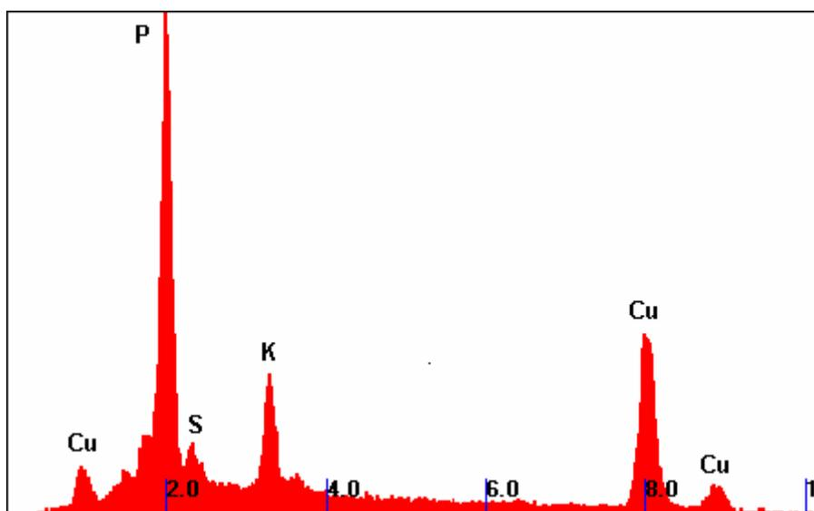
Coalescence of Cu-K phosphate rosettes, column A, experiment 2 pre- $\text{Ca}(\text{OH})_2$  addition. Note absence of Ca. Shown in Fig. 3.10b
