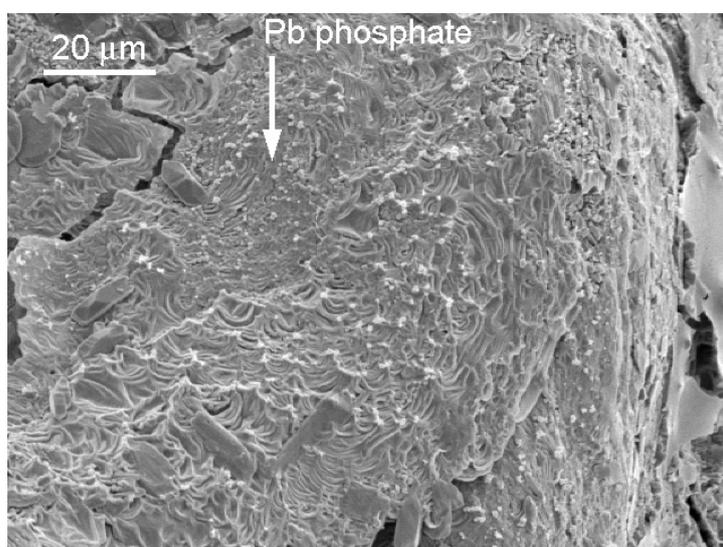
Scaly coating of Pb phosphate on galena, column D, post-coating stage, pre-Ca(OH)<sub>2</sub> addition.
