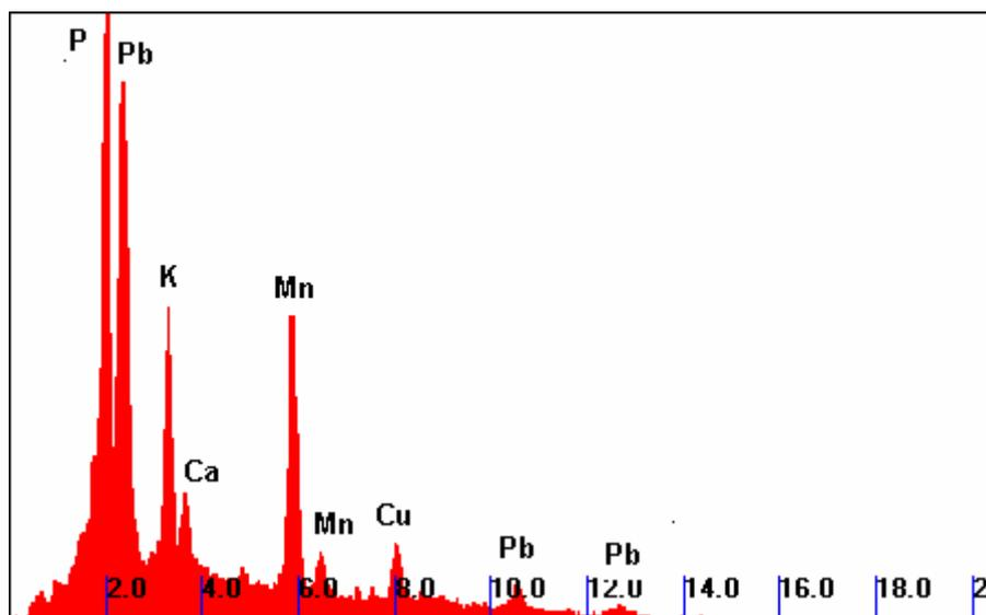
Globular Mn-K-Pb (Ca-Cu) phosphate coating, column A, experiment 3. Similar to material shown in Fig 3.16a.
