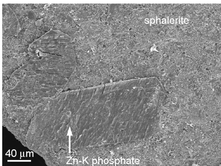
Large prismatic Zn-K phosphate crystals precipitated on otherwise uncoated sphalerite, column A, post-coating stage, pre-Ca(OH)<sub>2</sub> addition.
