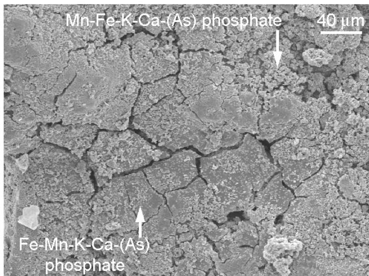
Granular Mn-Fe-Ca-(As) phosphate coating which becomes more amorphous with increasing Fe content, column E post-coating stage.
