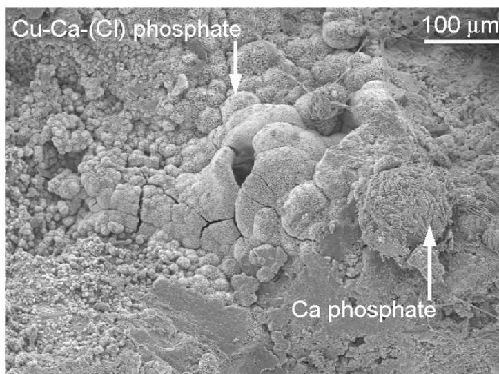
Botryoidal coalescence of Cu-Ca-(Cl) phosphate rosettes precipitated on quartz and chalcopyrite. Spherical Ca phosphate possibly a partially dissolved remnant fertiliser granule, column G post-coating stage.
