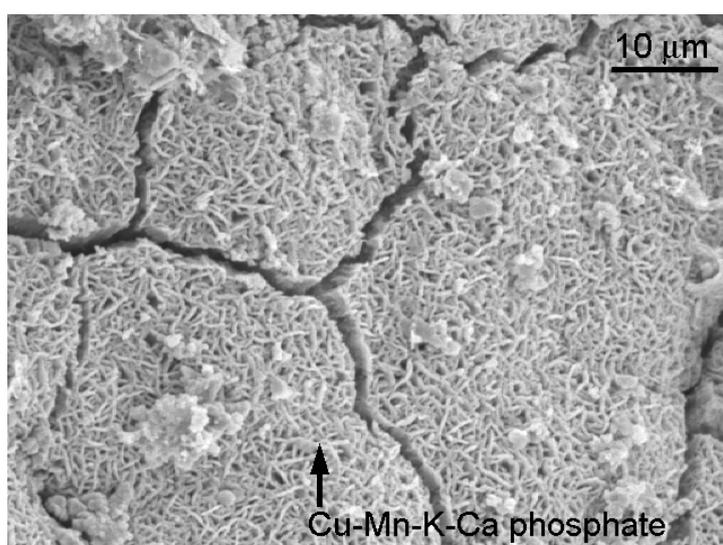
Detail of Cu-Mn-K-Ca phosphate coalescence showing desiccation cracks, column B post-dissolution stage.
