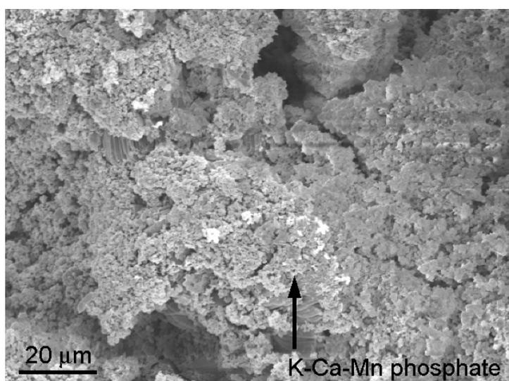
Granular K-Ca-Mn phosphate which forms the induration cementing grains together at the top of columns E and F (column E post-dissolution stage).
