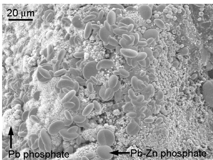
Bean-shaped Pb-Zn phosphate crystals precipitated on acicular Pb phosphate pincushions, column C post-dissolution stage.
