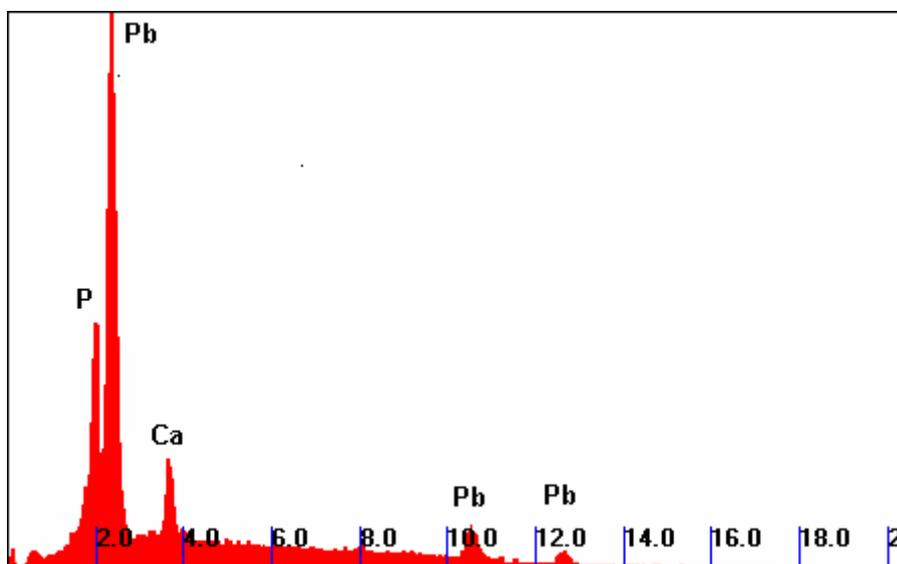
Pb-Ca phosphate, column D, experiment 1 post-coating stage.
