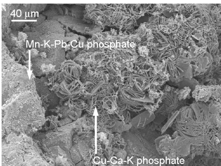
Spherical rosettes of Cu-Ca-K phosphate precipitated on Mn-K-Pb-Cu phosphate coating, column A post-coating stage.
