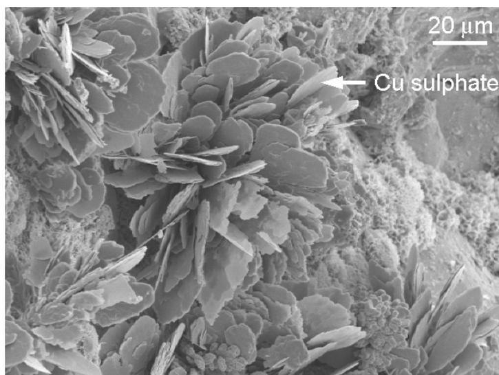
Cu sulphate rosettes, column D post-dissolution stage.
