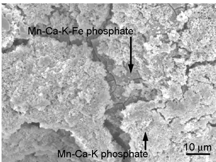
Coating of amorphous Mn-Ca-K-Fe phosphate with extensive desiccation cracks covered by precipitates of Mn-Ca-K phosphate, column F post-coating stage.
