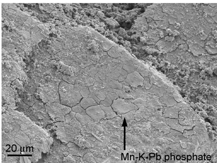
Coating of Mn-K-Pb phosphate on galena showing extensive desiccation cracks, column A post-coating stage.
