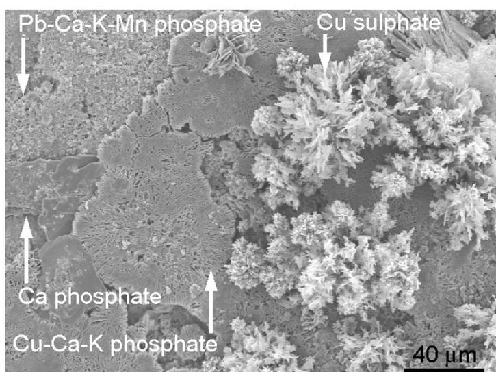
Cu sulphate rosettes precipitated on coalesced Cu-Ca-K phosphate rosettes which are precipitated on prismatic Ca phosphate crystals and Pb-Ca-K-Mn phosphate coating, column E post-coating stage.
