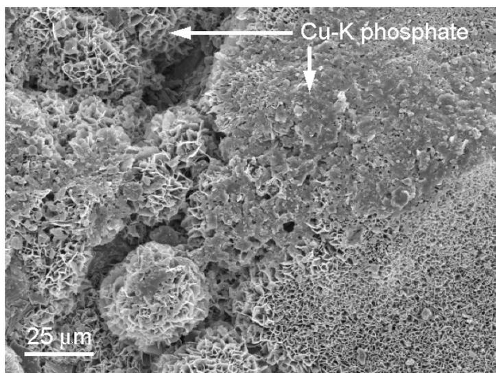
Detail of coalescence of Cu-K phosphate rosettes, column A, post-coating stage, pre-Ca(OH)<sub>2</sub> addition.
