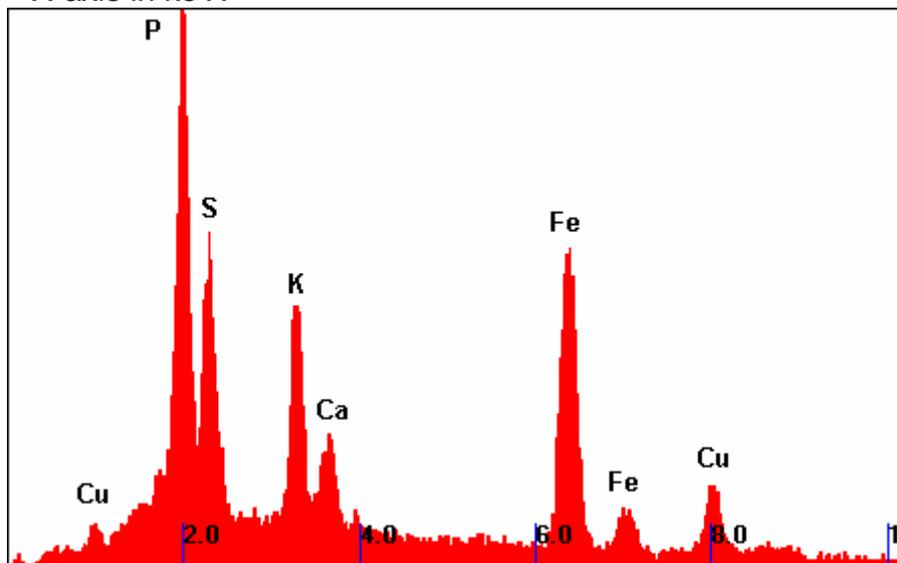
Fe-K-Ca-(Cu?) coating on chalcopyrite, experiment 1 post-coating stage. Similar to material shown in Fig 3.4a,b,d.
