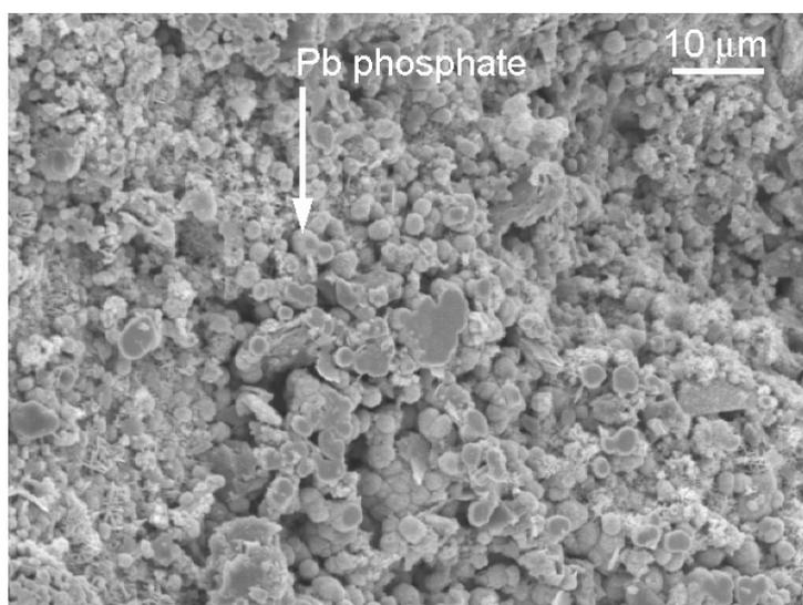
Granular to botryoidal Pb phosphates precipitated on galena, column D post-dissolution stage.
