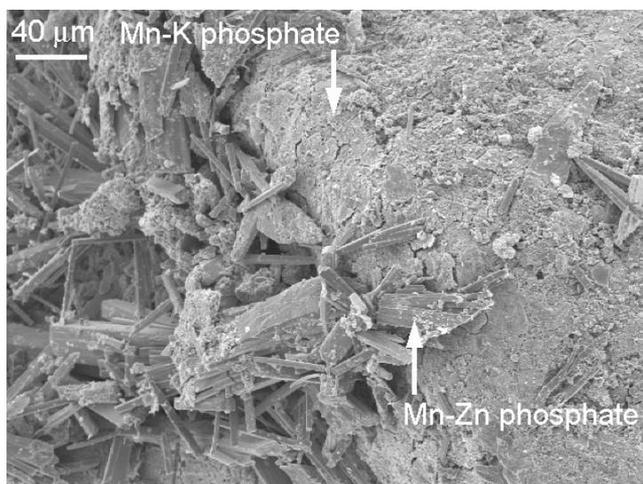
Prismatic Mn-Zn phosphate crystals precipitated on amorphous Mn-K phosphate coating with occasional desiccation cracks, column A post-dissolution stage.
