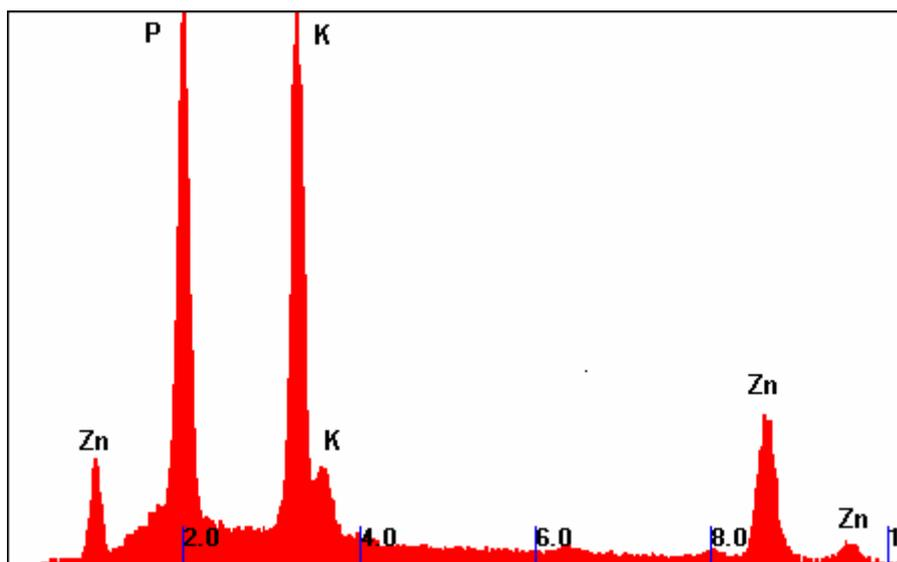
Flow-like Zn-K phosphate, column C, experiment 1. Shown in Fig. 3.4b and appendix B5
