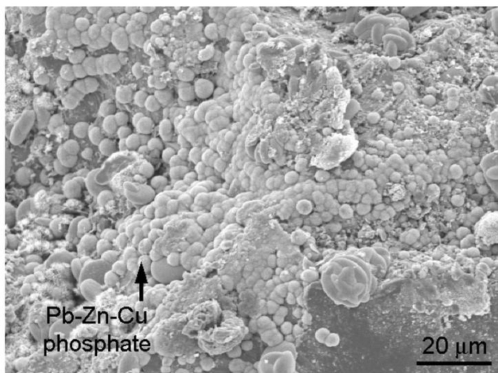
Botryoidal Pb-Zn-Cu phosphate precipitates on quartz, column C post-dissolution stage.
