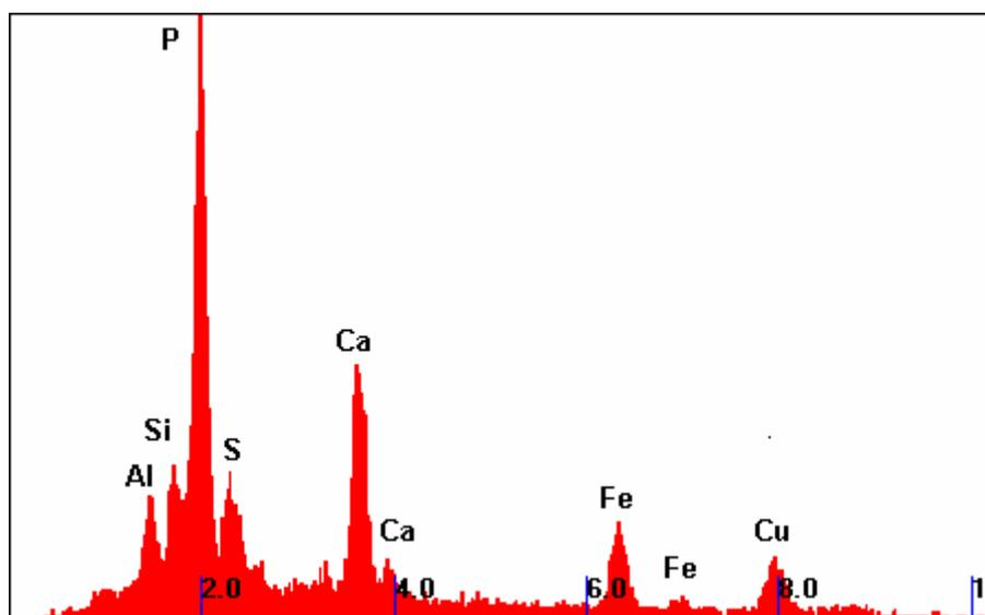
Granular precipitate of Ca-Fe-Cu-(Si-Al-S) phosphate, column G, experiment 3. Similar to material shown in Fig. 3.16c.
