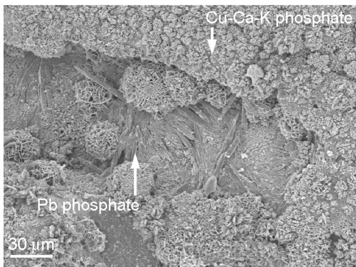
Tabular Pb phosphate crystals covered by calescence of Cu-Ca-K phosphate rosettes, column B post-dissolution stage.
