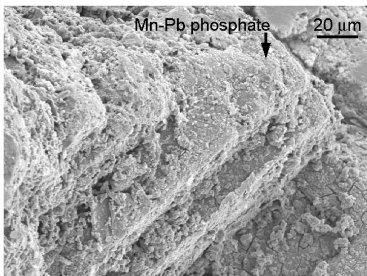
Globular to amorphous Mn-Pb phosphate coating on galena, column A post-dissolution stage.
