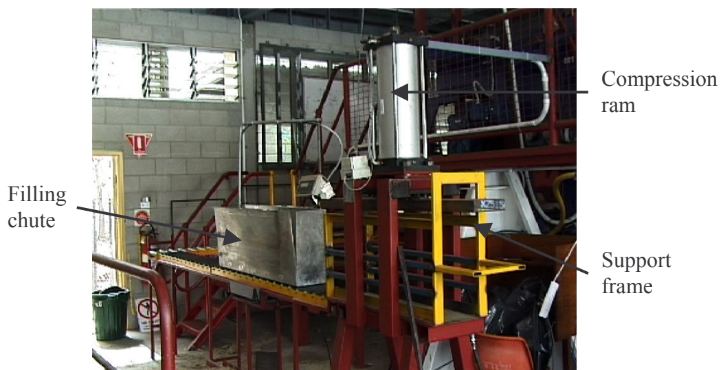
Figure 5.6. Pre-compressor used to prepare blankets for processing.
