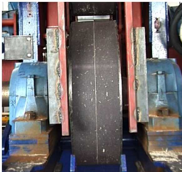
Figure 5.1. Flat rolls employed for the two-roll milling trials.
