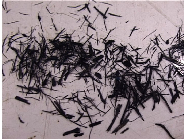
Figure 5.5. Material seed for enhancing contrast in experimental samples.
