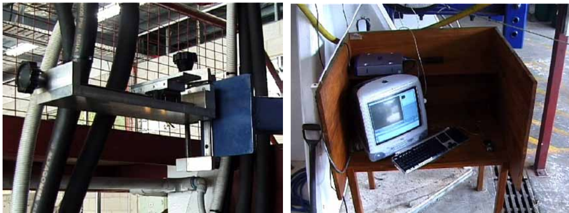
Figure 5.3. CCD traversing system and image acquisition apparatus.
