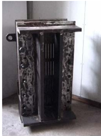
Figure 4.38. Thick blanket uniaxial cell with fitted viewing window.
