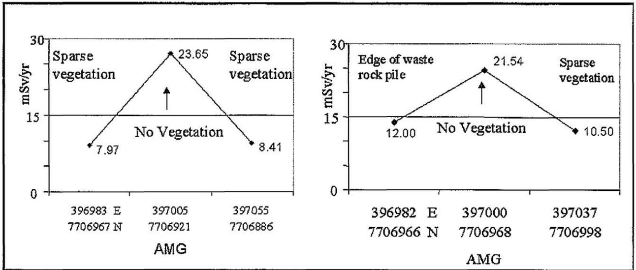
Traverse thirteen and fourteen surveyed the top of the D Stockpile. Radiation maxima occur on exposed waste rock (23.65 mSv/yr and 21.54 mSv/yr) and minima where waste rock is covered by soil and sparsely vegetated areas.
