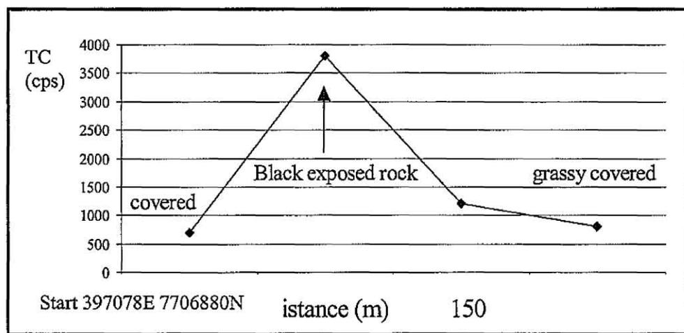
Traverse eight is also across the top of the North Waste Tip (bearing 100°). The maximum TC (3800 cps) reading was recorded on exposed ore and minimum readings (700 cps) were measured on areas where waste rock is thinly covered with ripped soil and sporadically grassed areas.
