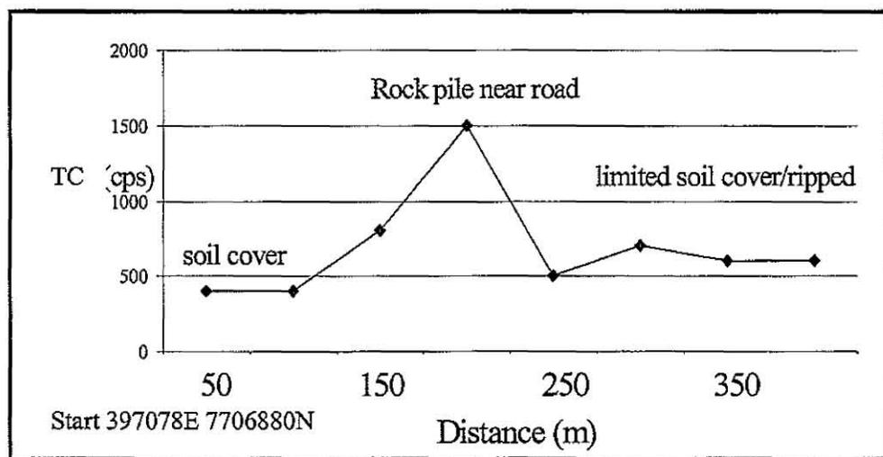
Traverse seven surveyed across the top of the North Waste Tip (bearing 10°). The maximum total count (1500 cps) reading was recorded on the waste rock pile toe, and minimum readings (400 cps) were measured on areas where waste rock is covered with soil. Soil cover that is ripped, provided less radiation dampening than full soil cover (total count 500 cps - 700 cps).
