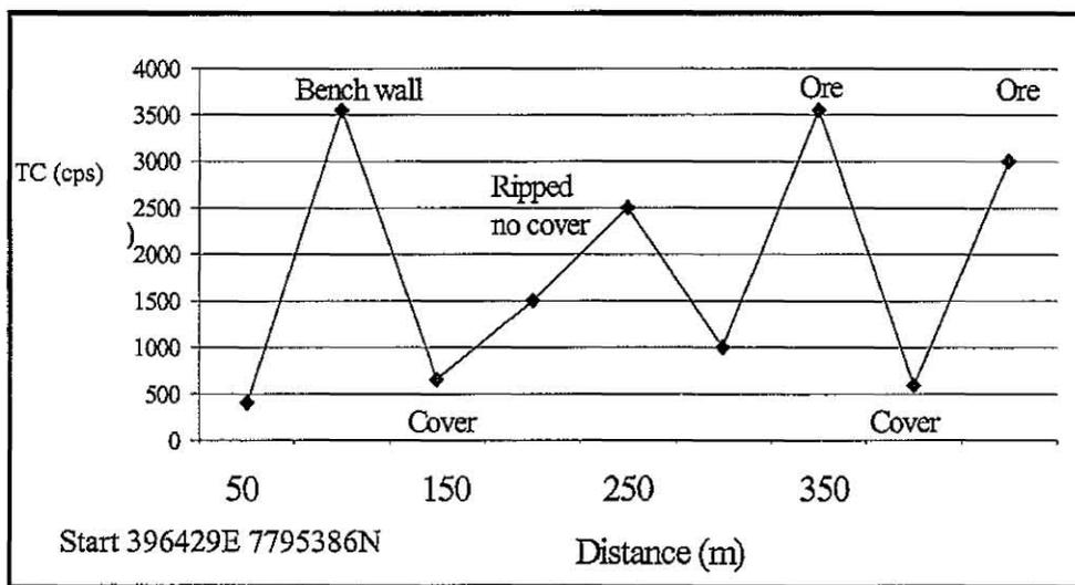
Traverse 3 is also across the West Tip (bearing 35°). It started on soil covered waste rock, continued to the bench wall (made of waste rock) and traversed across exposed and non exposed waste rock areas. Maximum total count (3550 cps) readings were recorded on exposed rock boulders, these high readings indicate that these rocks contain uranium ore. Minimum readings (400 cps) were measured on soil topped surfaces.
