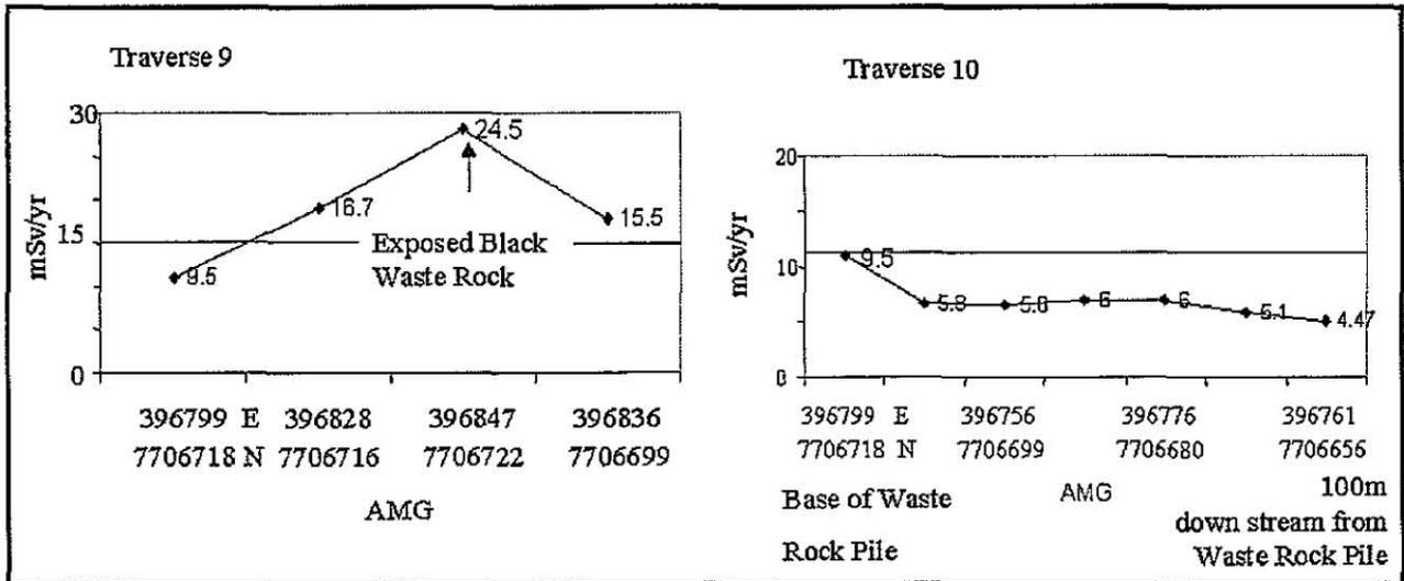
Traverse 9 measured around the base of the Crusher pile with maximum radiation at (24.5 mSv/yr) where ore was exposed. Traverse 10 started at the base of the Crusher pile and followed the drainage channel away from the waste rock pile. Maximum radiation at (9.54 mSv/yr) was at the toe of the waste rock pile and decreased significantly away from the pile (to 4.47 mSv/yr).
