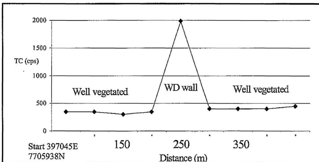
Starting on the concrete foundation (Bearing 0°) near the base of the Crusher pile, the survey traversed the waste rock wall and continued to another well vegetated area. A maximum total count (2000 cps) reading was recorded on the bench wall, and minimum readings (300 cps) were measured on areas away from waste rock piles.
