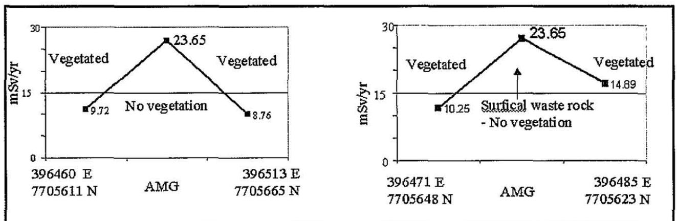
Traverse eleven and twelve intersect on the West Tip at the maximum reading of 23.65 mSv/yr, which also corresponds to the area with no soil or vegetation cover.
