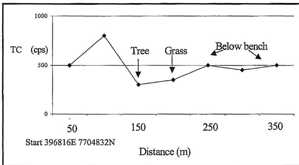
Traverse one across the South Waste Dump starts over exposed waste rock, continues to soil covered areas with established vegetation and ends on exposed waste rock. Maximum total count (800 cps) values were recorded on exposed waste rock and minimum (300 cps) values on vegetated surfaces.
