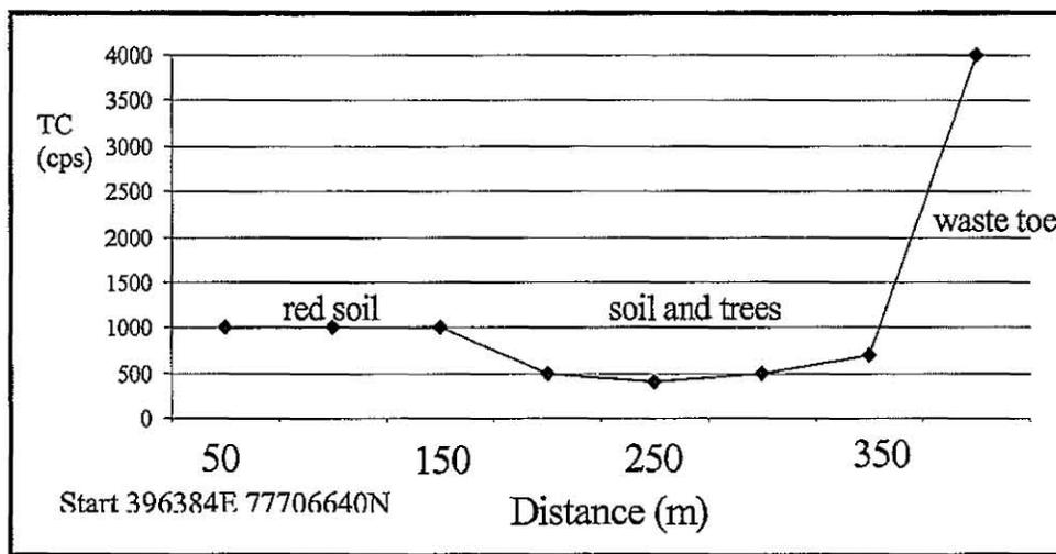
Starting below the Crusher pile around mill site (Bearing 80°) the survey headed toward the waste pile toe. Maximum total count (1000 cps) readings were recorded on the waste rock pile toe, and minimum readings (400 cps) were measured on areas away from the waste rock pile. The area noted as red soil (poorly vegetated) within the old mill/processing site had elevated readings (1000 cps) and corresponds to MKS10.
