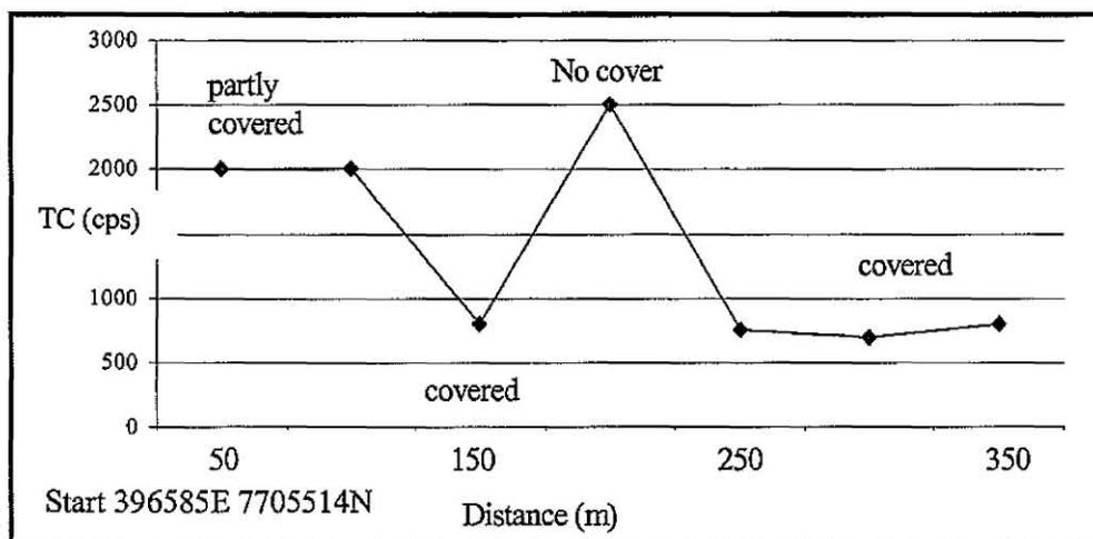
The survey of the West Tip top surface (bearing 250°) started on partially soil covered waste rock, continued across exposed and soil covered waste rock areas. Maximum total count (2500 cps) values were recorded on exposed waste rock and minimum (750 cps) values on soil topped surfaces.
