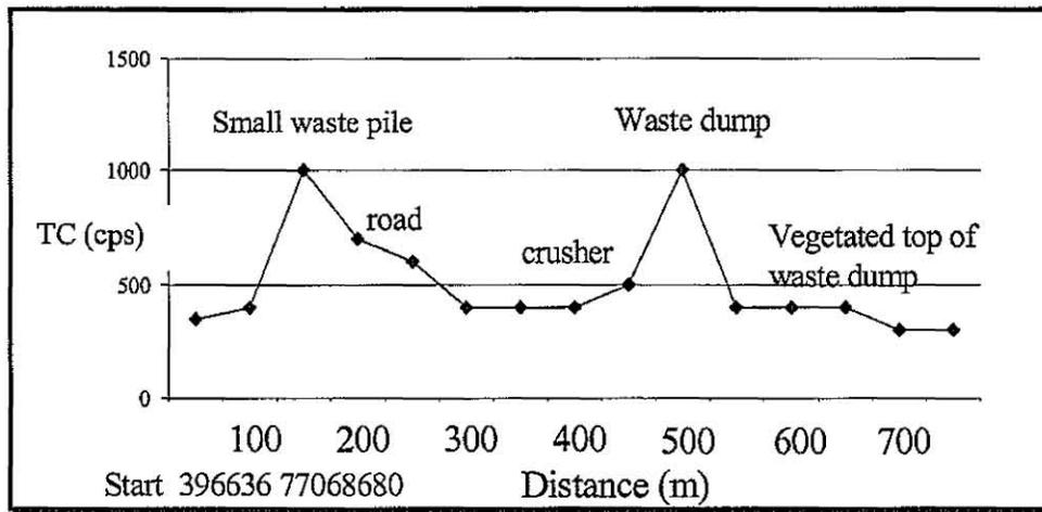
Traverse five started in the old processing area (bearing 180°), continued over the concrete foundation up the Crusher pile slope to the top of the dump. The maximum total count (1000 cps) reading was recorded on the waste rock pile slope, and minimum readings (300 cps) were measured on areas away from the waste rock pile and on the well vegetated top of the Crusher pile.
